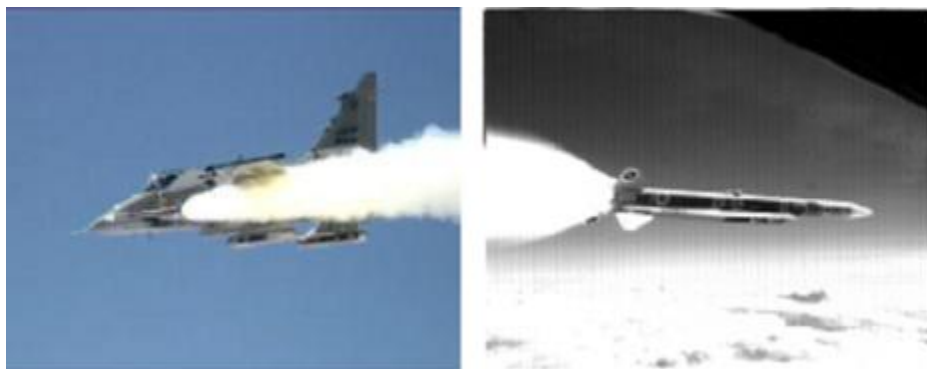
Figure 1: Meteor flight testing, launch and early boost phase (photos courtesy of MBDA Missile-Systems)
