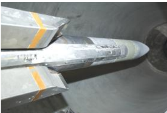
Figure 8: Meteor M2 development standard motor with forebody mounted in the Modane windtunnel (photo courtesy of MBDA)
