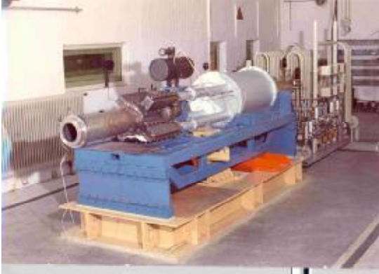
Figure 10: Experimental ducted rocket test motor (diam 240 mm), 1975
