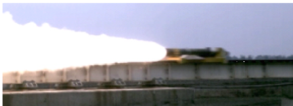
Figure 31: Sled test of the boost motor; 2005
