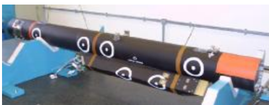
Figure 31: Meteor M2 development standard motor as delivered for flight testing
