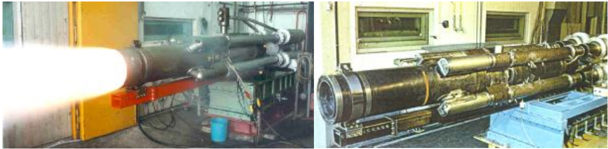
Figure 18: Testing of the TDR motor for ANS, left cp test, right semi freejet test; 1987
