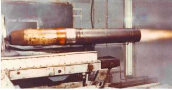
Figure 8: Windtunnel testing of a HYDRA fullscale engine pod
