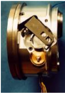
Figure 22: DEM interstage/control valve assembly
