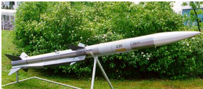
Figure 23: EURAAM missile with flightweight TDR motor
